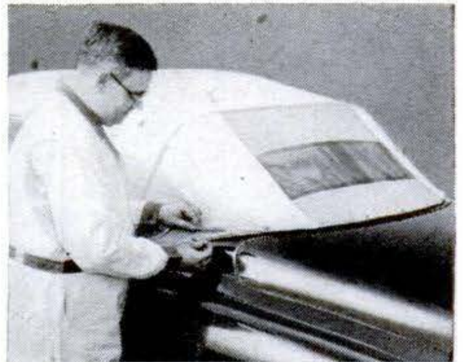
RAIN COVER. Studebaker-convertible owners can slip a water-repellent fabric cover, with a transparent rear curtain, over the regular top. The top can be raised and lowered without removing the cover.
